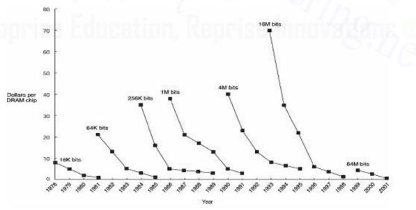
Between the start of a project and the shipping of a produce, say, two years, the cost of a new DRAM drops by a factor of between 5 and 10 in constant dollars.
